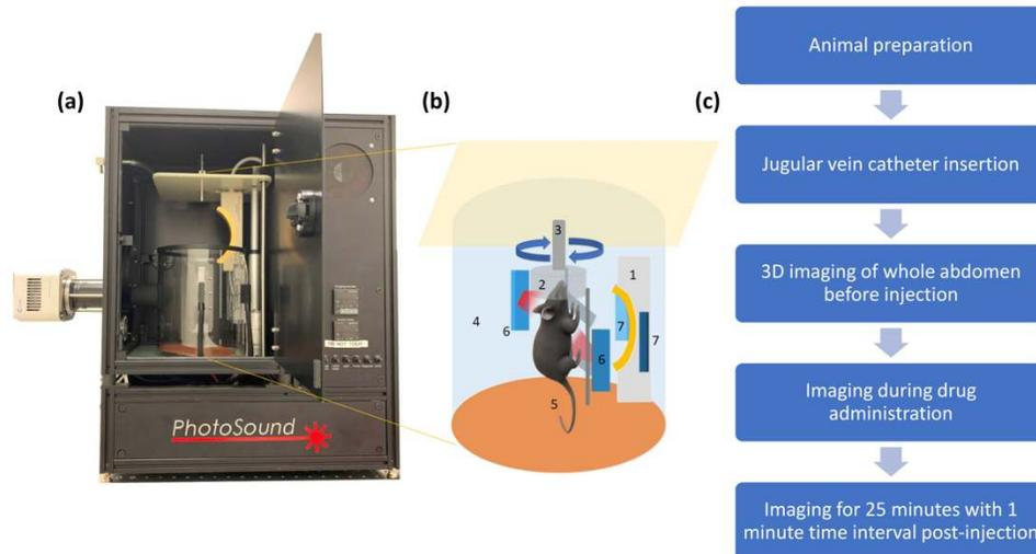
Figure 1. (a) A photoacoustic tomography system (TriTom). (b) A schematic diagram of photoacoustic tomography system. (1) Arc array transducer, (2) Animal holder with nose cone, (3) Anesthesia tube, (4) Imaging chamber, (5) Heating pad, (6,7) Optical fiber terminals. (c) Flow chart of experimental method.
