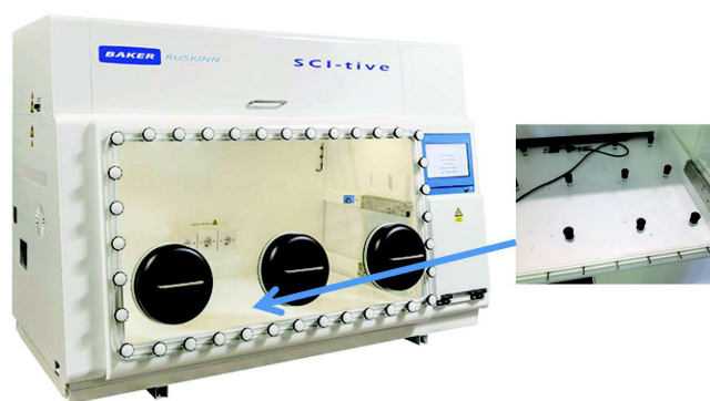
Figure 1. SCI-tive (left) with inset showing ferrules that support the internal floor tray (right)
