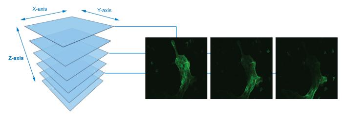
Simply position the probe once and through the use of the interactive and continuously variable depth control (z-axis) you can capture all of the images you need as Optical sections and generate 3D visualisations that allow you to study and analyse your discovery.
