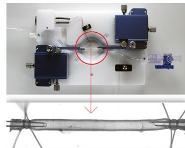
A digital camera connected to a microscope is positioned above the vessel chamber where the inner/outer diameters and wall thicknesses of the vessels are digitized and quantified. It is the changes in these dimension that are the direct measure of vessel reactivity.
