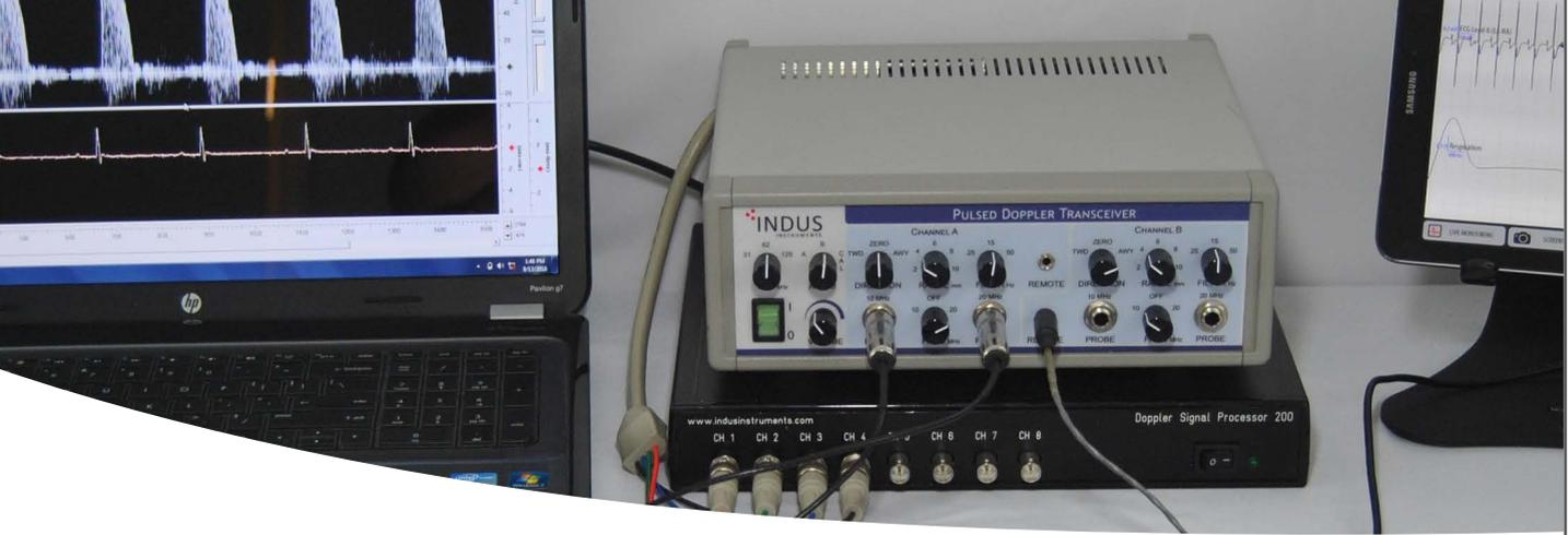
**The Doppler Flow Velocity System** is a high-frequency, real-time pulsed Doppler measurement device with integrated data analysis software designed specifically for measuring cardiovascular function in small animals. The high sampling rates grant excellent temporal resolution, making this the ideal system for studying fast heart rates and rapid blood accelerations present in mice and other small animals. No imaging required.
